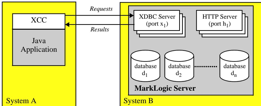
As shown in the diagram above, the XCC-enabled application can run on the same system as an instance of MarkLogic Server (a host), or it can run on a completely different system, as long as the two systems are networked together.
