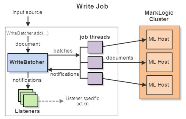
The following diagram gives an overview of the key components and actions of a write job:
